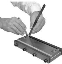
NOTE: The knives must butt up against the rings on the outer edges of the cutter housing.
